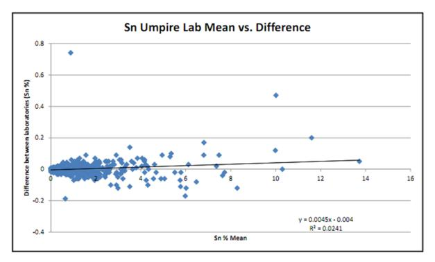
Figure 3-17 Umpire lab precision pairs plot (difference vs. mean)
