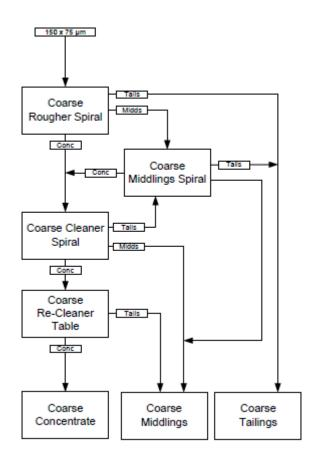
Figure 6-19 Coarse gravity separation
