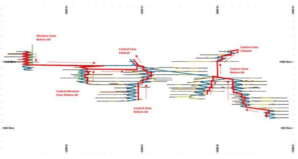
Figure 5-44 Achmmach mine plan return air route (red)
