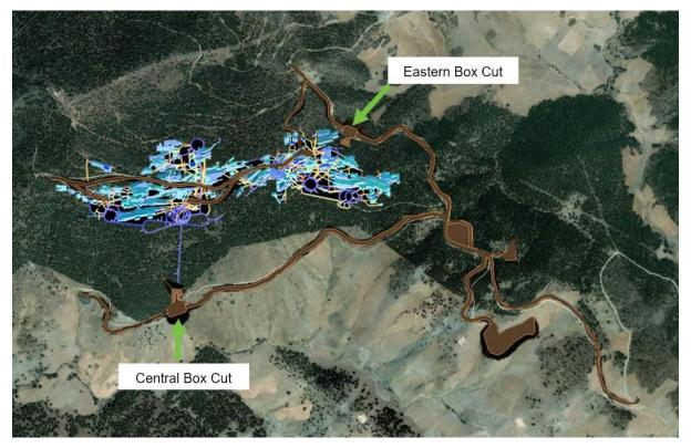
Figure 4-32 Surface layout showing central and eastern box cut positions
