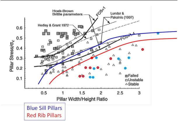
Figure 4-24 Comparison between Achmmach pillar and industry designs.
