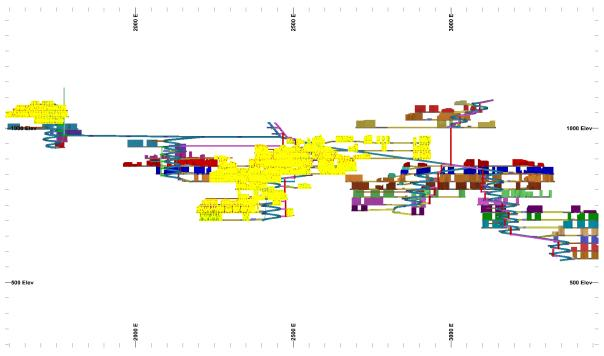
*Figure 5-5 Mining methods by zone, CRF highlighted yellow otherwise top down with pillars*
