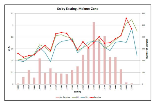
Figure 3-35 Swath Plot for Meknès Zone by Easting
