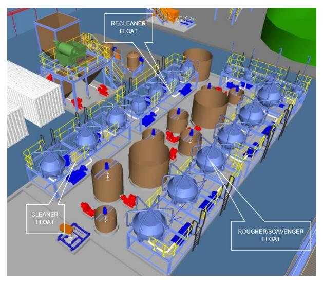
Figure 6-21 Flotation circuit
