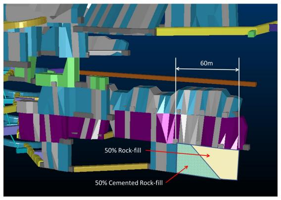
Figure 4-29 Modified Avoca using CRF.
