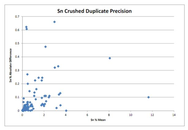
Figure 3-25 Sn Original vs. coarse crush duplicate precision chart
