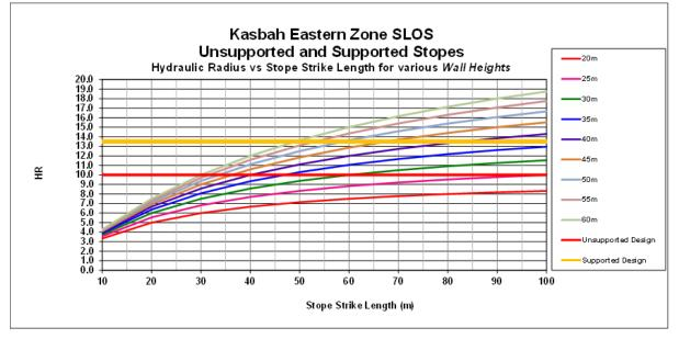
Figure 4-23 Eastern Zone-Design guidelines for stable unsupported and supported walls.
