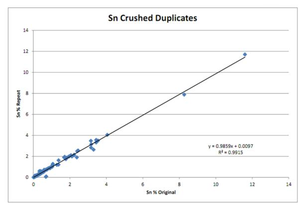
Figure 3-24 Scatterplot Sn Original vs. Coarse Crush Duplicate
