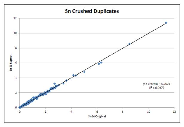
*Figure 3-14 Scatterplot Sn original vs. coarse crush duplicate*
