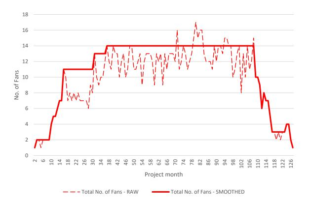
Figure 5-49 Operating auxiliary fan schedule (110 kW)
