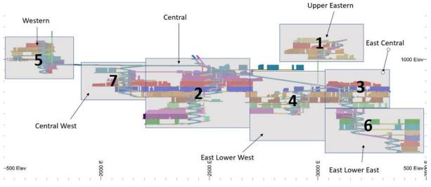
*Figure 5-29 Achmmach mine plan mining sequence (long section looking North)*
