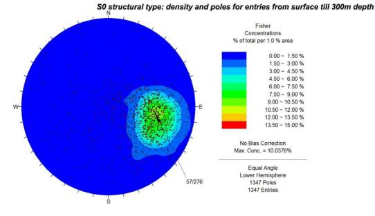
Figure 4-8 Distribution of bedding and foliation surface to 300m depth
