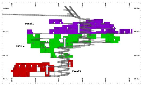
Figure 5-3 Central zone schedule showing concurrently mined panels (long-section looking north) (coloured by panel)
