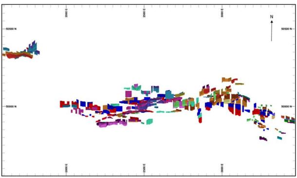
Figure 5-9 Plan view stope design (coloured by RL)
