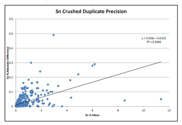
Figure 3-15 Sn original vs. coarse crush duplicate precision chart
