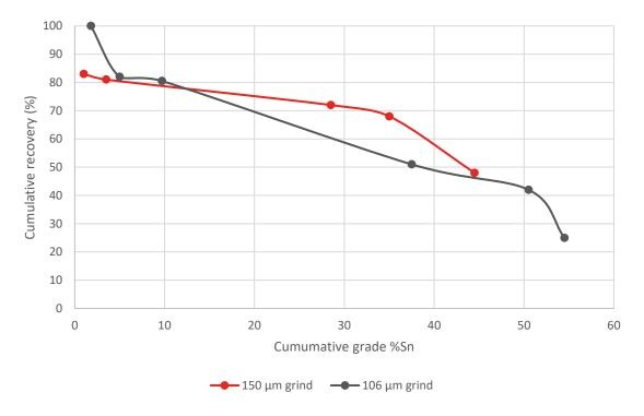
Figure 6-5 Grade recovery comparison for grind size
