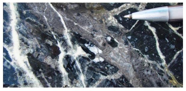
Figure 3-7 Fine grained cassiterite (brownish) as vein infill and dissemination along the edges with late stage cross cutting carbonates (whitish) veins
