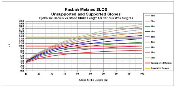
Figure 4-21 Meknès Zone-Design guidelines for stable unsupported and supported walls.
