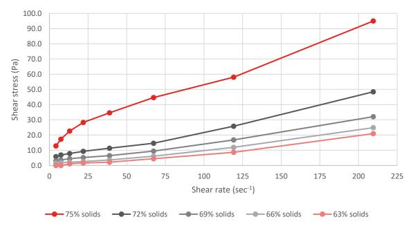
Figure 6-7 Shear stress Vs shear rate
