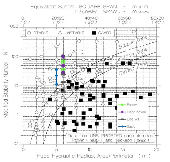
Figure 4-19 N' vs HR values for the unsupported stopes East Zone (Hutchinson & Diederichs 1996)
