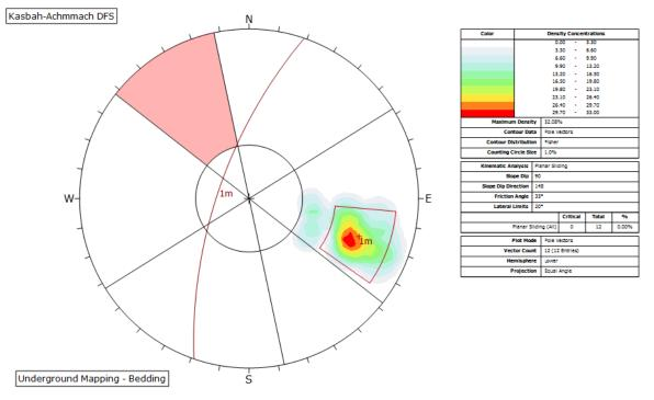
Figure 4-35 Plane failure in the portal high wall central boxcut
