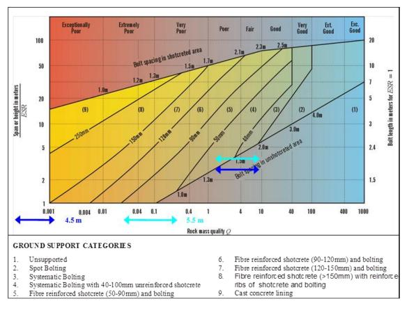
Figure 4-41 Civil engineering approach (based on Q)
