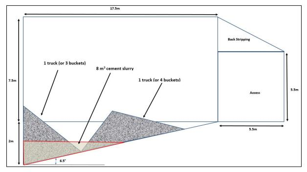
Figure 5-24 Long-section schematic of stockpile mixing cuddy (not to scale)
