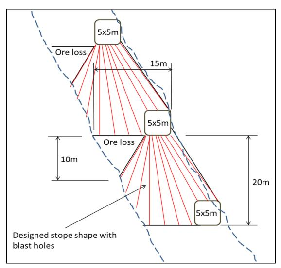
Figure 4-30 Cross-sectional view of stope design when using Avoca for wide orebodies.
