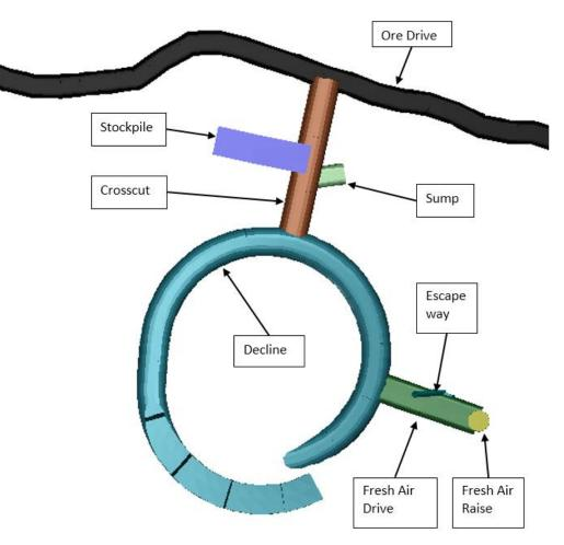
Figure 5-11 Typical level layout-plan
