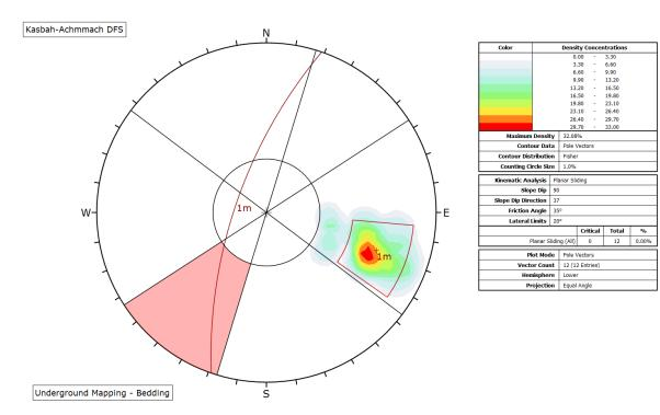
Figure 4-34 Plane failure in the portal high wall east boxcut
