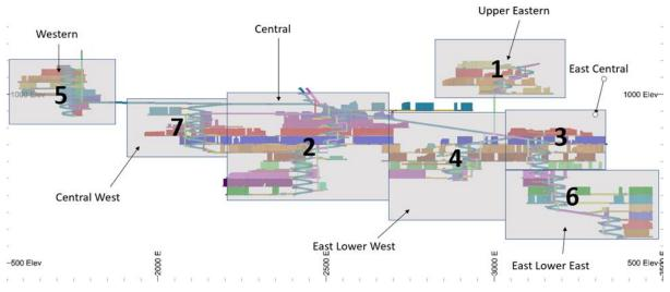
Figure 1-6 Mining sequence (long section looking North)
