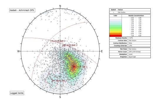
Figure 4-10 Joint sets logged data
