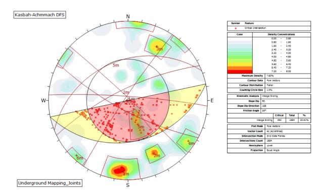
Figure 4-39 Wedge failure in the portal high wall west
