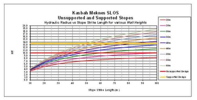
Figure 4-20 Meknès Zone-Design guidelines for stable unsupported and supported backs.
