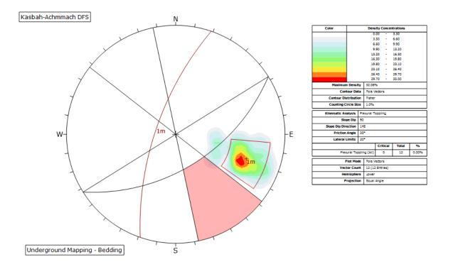
Figure 4-37 Toppling failure in the portal high wall central boxcuts
