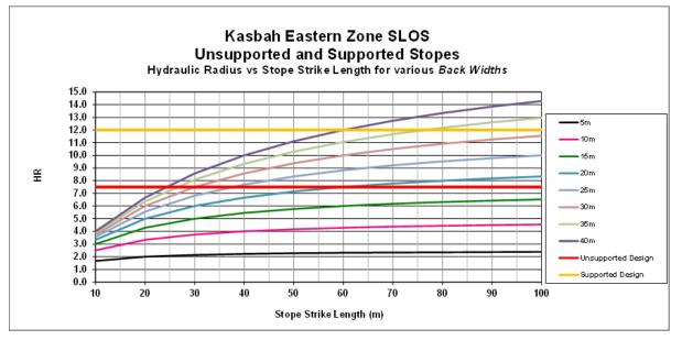
*Figure 4-22 Eastern Zone-Design guidelines for stable unsupported and supported backs.*
