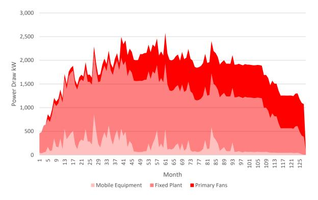
Figure 5-51 Peak power draw estimate over life of mine in kW
