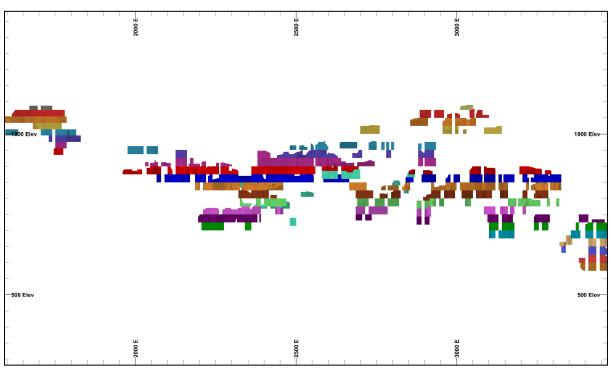
Figure 5-8 Long-section stope design (looking north coloured by RL)
