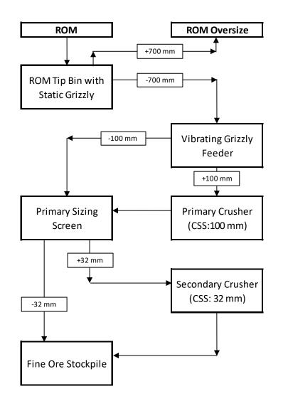
Figure 6-17 Crushing circuit flow diagram
