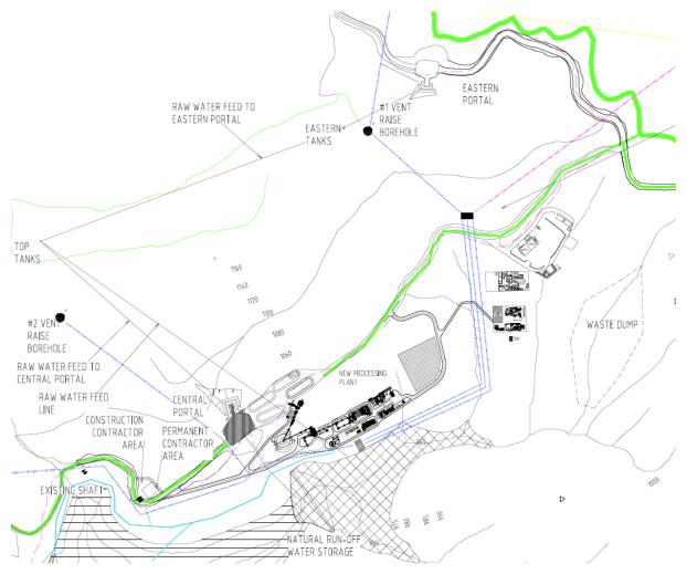
Figure 5-13 Portal layout in relation to key surface infrastructure
