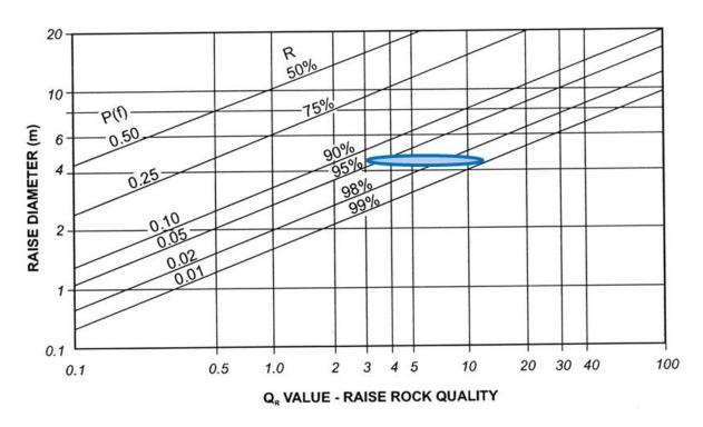
Figure 4-46 Risk ratings for the raise bore shafts (Diameter 4.5m)
