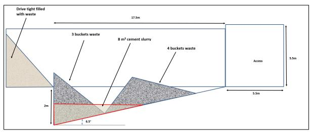
Figure 5-25 Long-section schematic of inactive drive mixing cuddy (not to scale)
