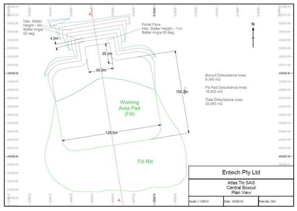
Figure 5-15 Plan view of central boxcut and apron
