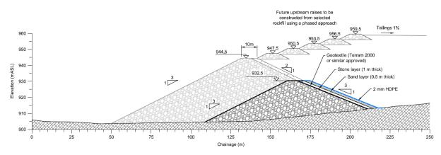
Figure 7-1 TSF typical embankment section
