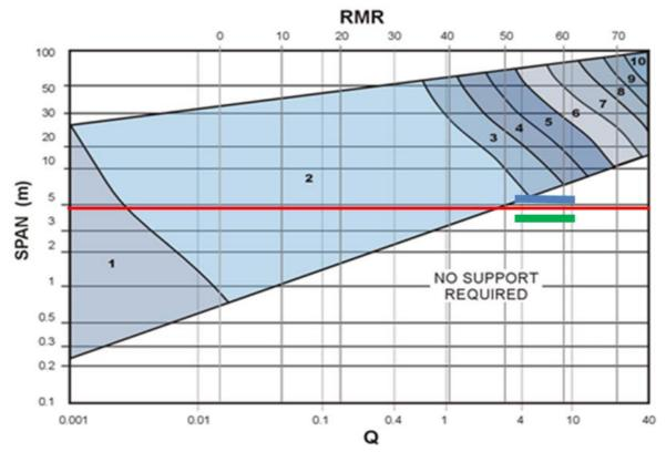
Figure 4-42 Mining approach for rock bolts (based on RMR)
