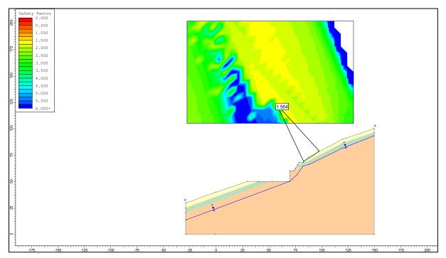
Figure 4-40 SLIDE model for the central and east box cut (FoS = 1.55)
