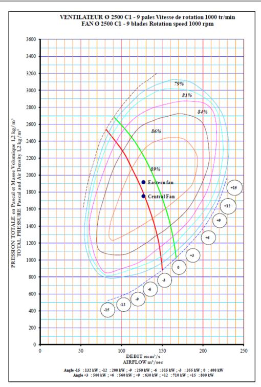
Figure 5-46 Fan curves for proposed primary ventilation system
