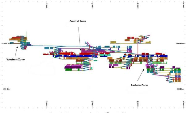
Figure 1-4 Long section showing different mining zones
