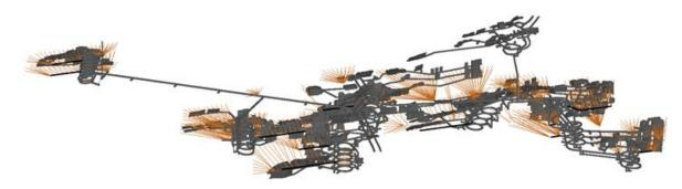
Figure 5-41 Designed grade control program (isometric view looking NE, diamond drill drives shown black)
