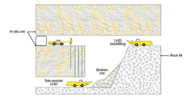
Figure 4-28 Schematic showing typical Avoca method.
