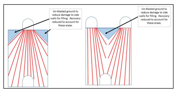
Figure 5-22 Ore recovery loss in wide bottom-up stopes
