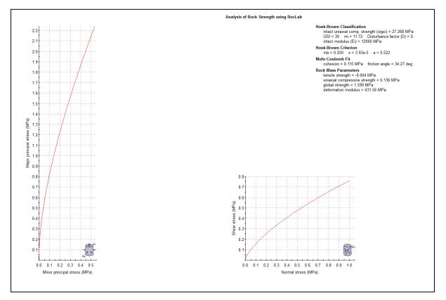
Figure 4-5 Rock Strength Analysis for the Weathered Rock
