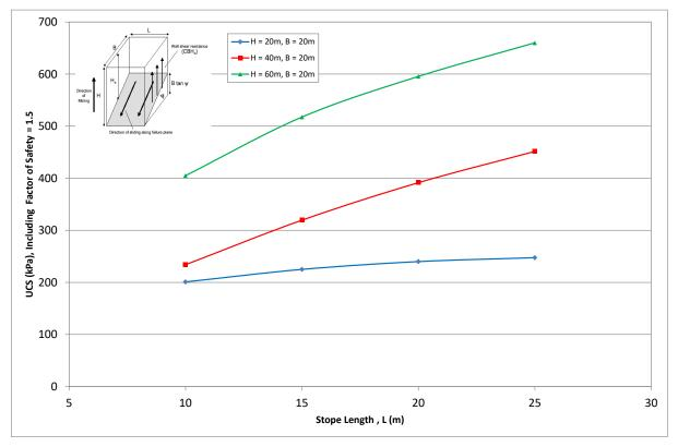
Figure 4-27 Analysis of CRF exposure stability.
