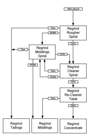
Figure 6-20 Regrind gravity separation
