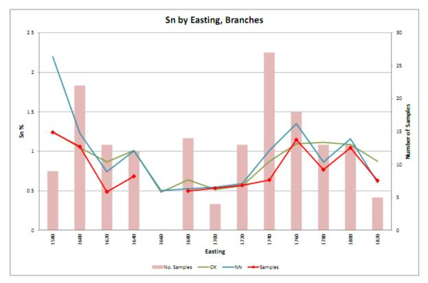
Figure 3-44 Swath plot branches by easting
