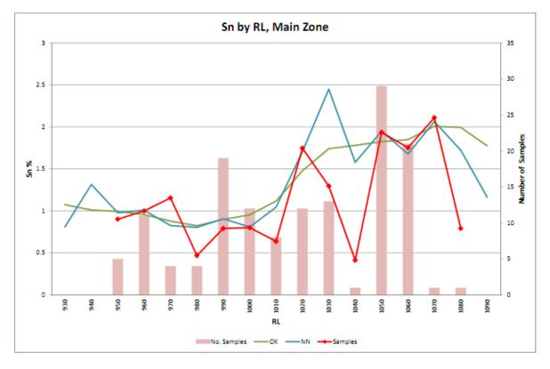
Figure 3-43 Swath plot main zone by RL
