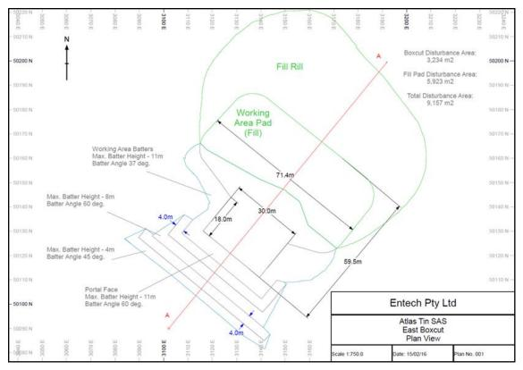
Figure 5-17 Plan view of eastern boxcut and apron
