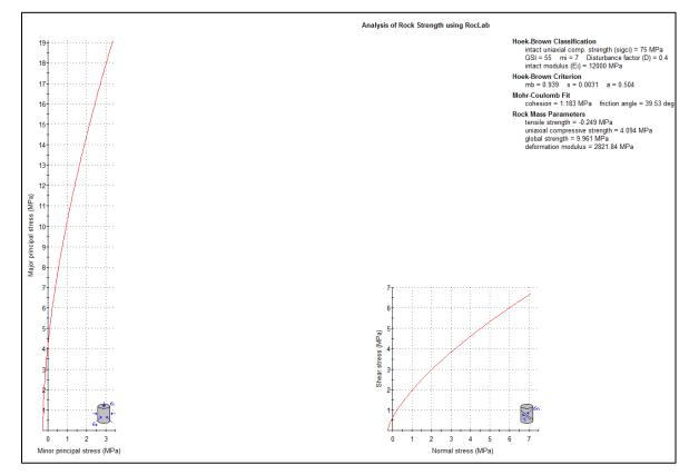
Figure 4-4 Rock Strength Analysis for the Hard Rock
