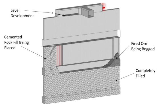
Figure 5-26 Bottom-up CRF mining method
