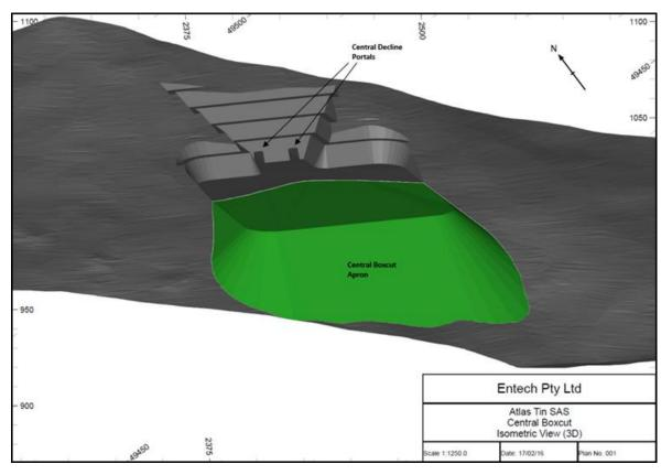
Figure 5-14 Isometric view of central boxcut and apron (looking NE)
