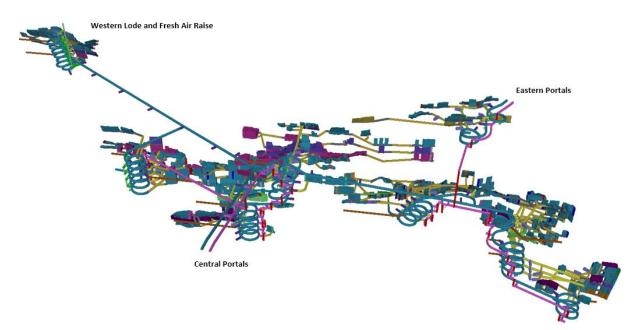
Figure 1-3 Isometric view of development and stope design
